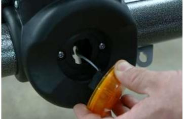
**Step 6:**Pull wiring out of tongue from rear of tongue underneath deck of trailer
