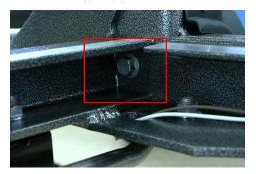
**Step 13:**Remove yoke bracket bolts (4) from side frames
