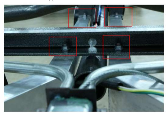
**Step 11:** Remove bolts from yoke side brackets from side frames
