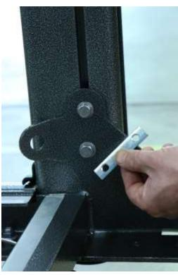
**Step 12:** Remove lift tube bolts (2) through yoke and side frames
