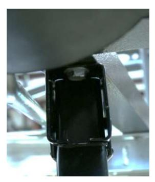
**Step 10:**Remove bolts and nuts (4) from c-channels
