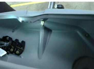
**Step 2:**Remove damper (shock) from yoke
