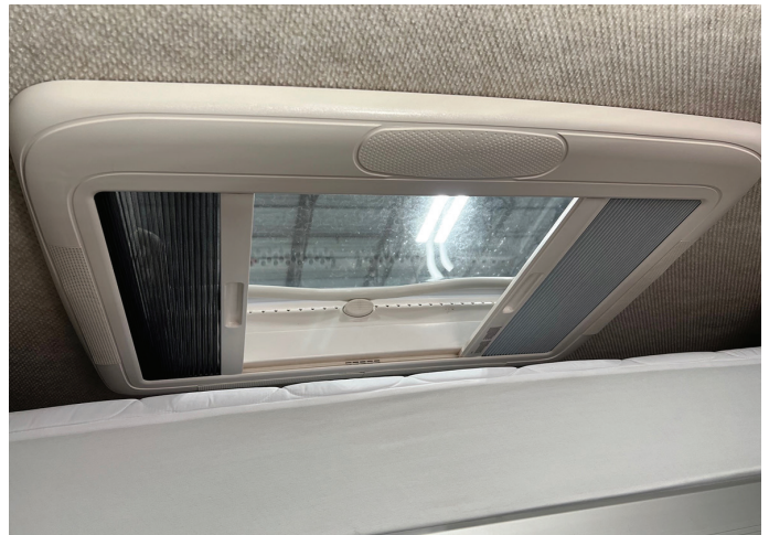
Skylight, with shade and blackout curtain
