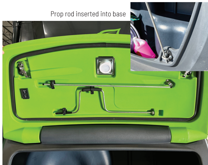
Lockable front storage box lid contains prop rod, jack handle, tap light and wireless light switch
