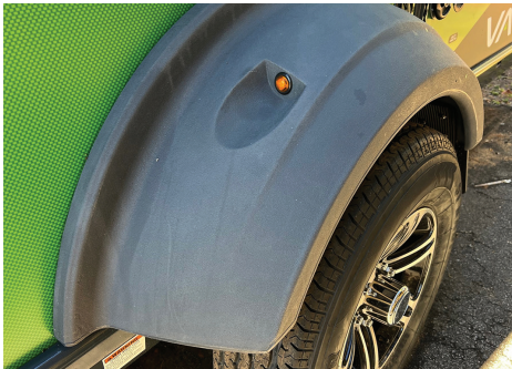
Fender LEDs, red (rear) and amber (front, shown)
