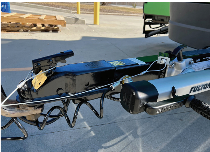
Hitch and safety cables, breakaway cable connected to tow vehicle
