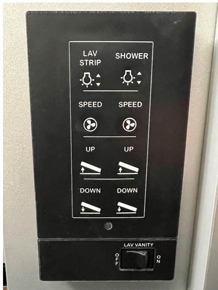
Wireless switch panel, located in bathroom
