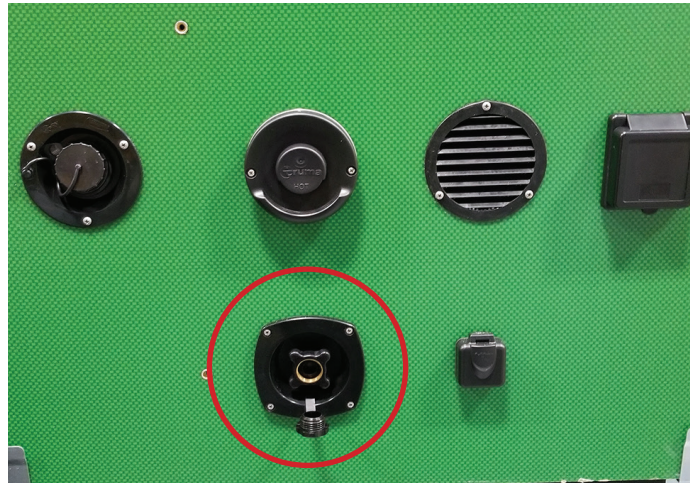
Fresh city water connection circled in red
