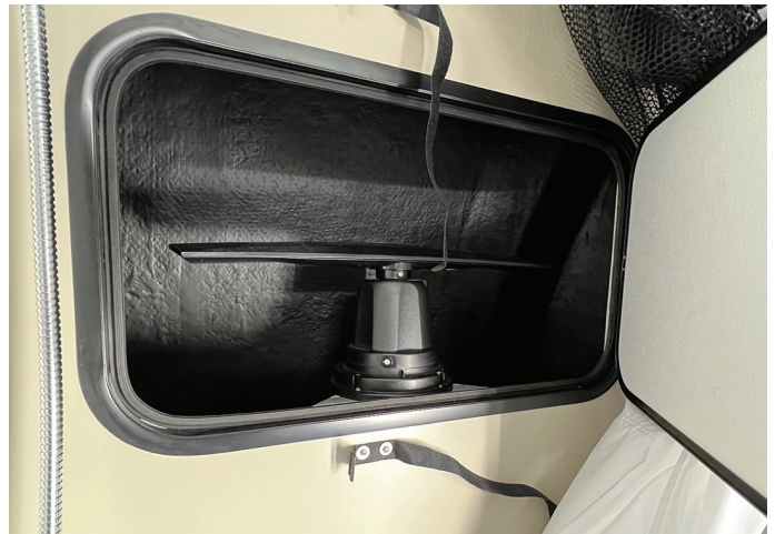
WiFi antenna mounted inside front cap, with access door inside
