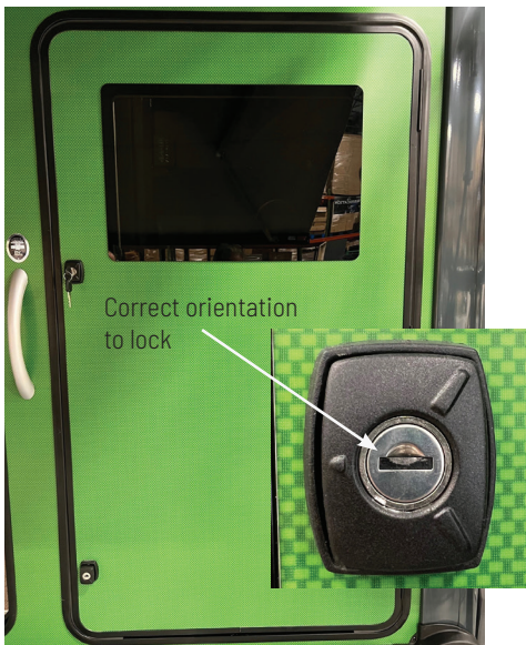
Kitchen access panel - closed and locked
