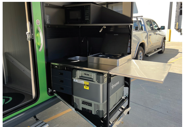
Kitchen in outside position
