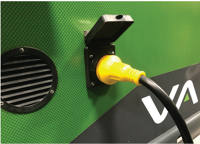
Shore power connection
