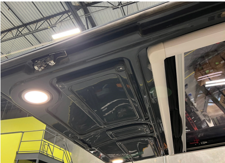
Lift gate lights
