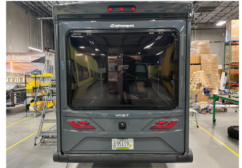
Rear stop/tail/turn lights and center high mount
