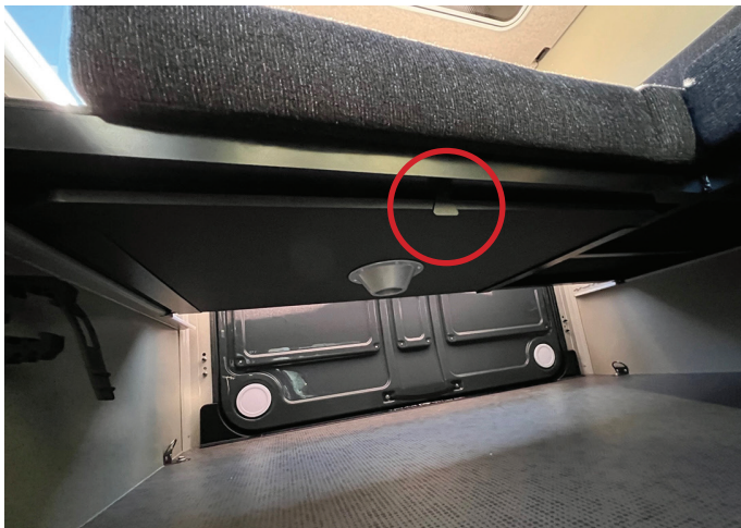
Dining table located on storage shelf underneath movable lounge. Release tab shown circled
