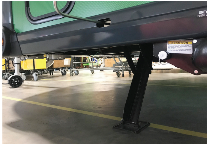
Rotate crank handle to raise and lower leveling jacks
