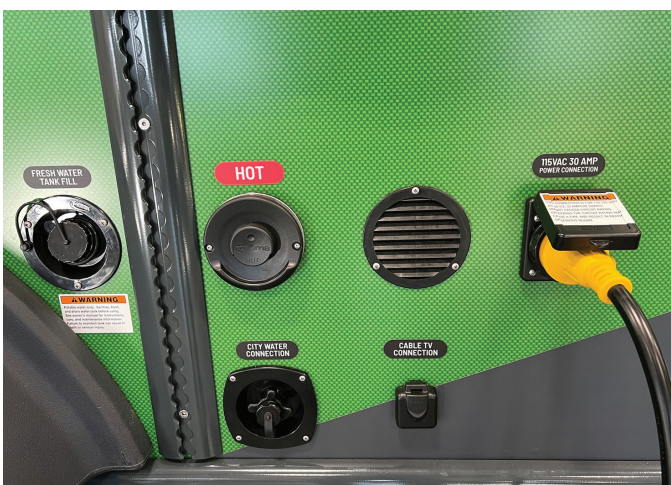
Facilities ports and vents
