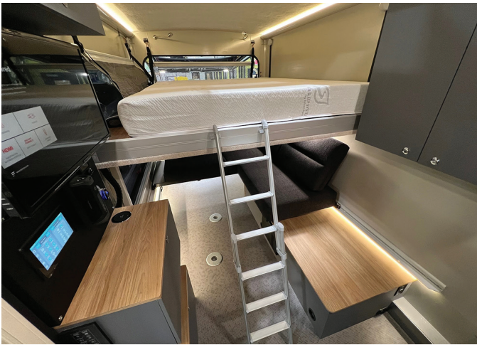
Bed lowers from ceiling and has ladder for access
