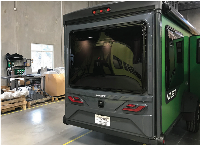
Lockable rear door, with lift assist
