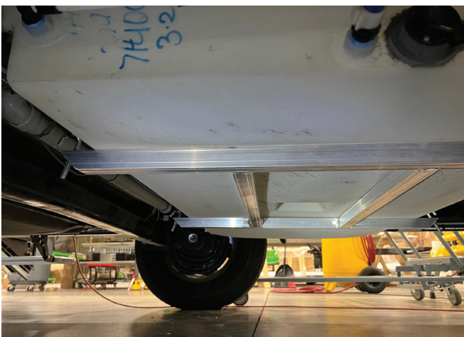
Fresh water tank, view from underneath
