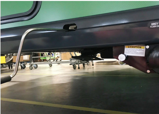
All four leveling jacks have access slots for crank handle
