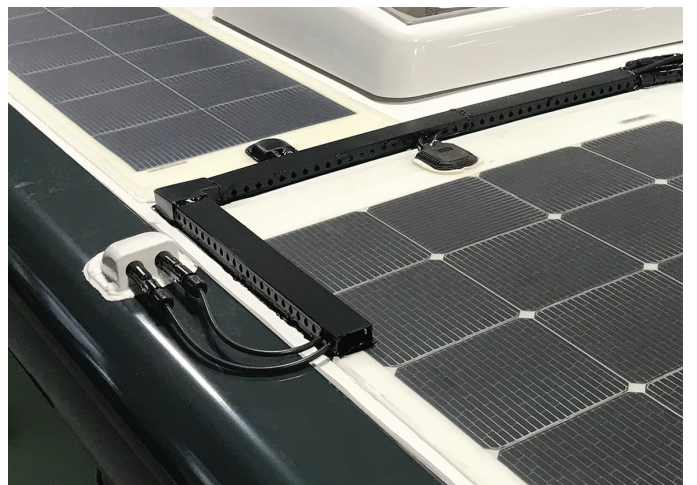
Solar panel connections and cable routing
