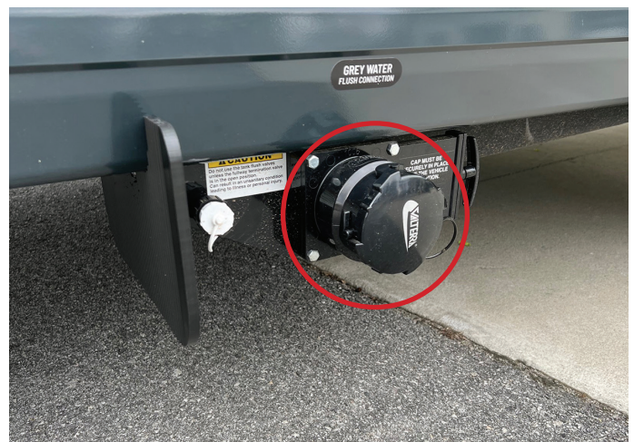
Gray water tank and flush port (circled), view from underneath
