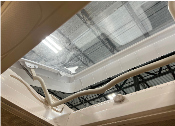
Skylight, push button to unlock, move grab bar to set position
