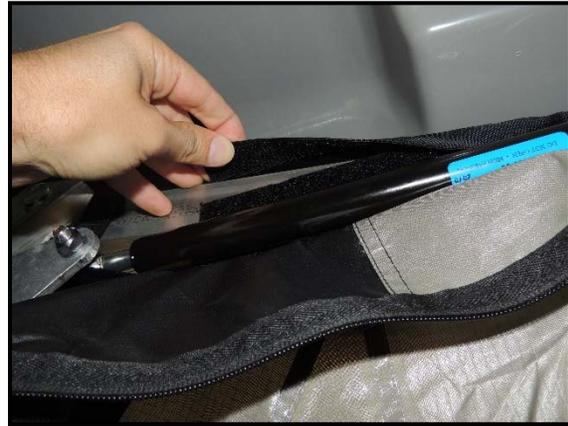
**Step 12:** Unfasten the long webbing (yellow) that the tent is hanging from and connected to the outer flap and wrap it around the front of the rectangular tube (B) and attach to the Velcro sleeve as shown (captured between the two layers).
