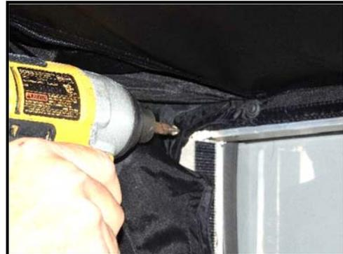
**Step 4:** Detach the flaps around the ceiling of the tent. Finally, unclip the two upper corners and remove the old tent from the trailer.
