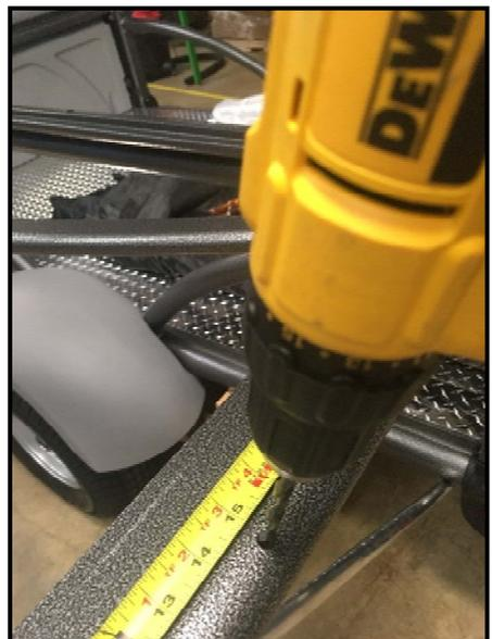
**Step 25:** Drill each hole and, if necessary, remove any sharp edges from around the hole with a file.
