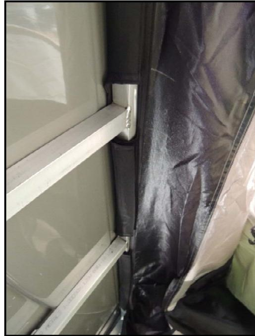
**Step 16:** At the bottom of the front wall loop the small Velcro straps around the bottom cross bar and secure loosely as shown.
