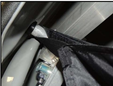
**Step 8:** Locate one of the upper, rear buckles and loop the male end over the rod at the rear corner of the tent pod as shown.
