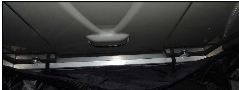
**Step 17:** Attach the bottom flap to the Velcro on the lower front wall.
