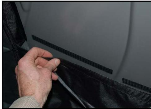
**Step 18:** Attach the upper flap to the Velcro on the top crossbar and on the sides of the triangular frame brackets as shown.
