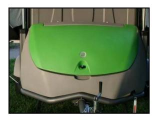
If the gap between the lid and the front storage box is too large it can be adjusted easily.
