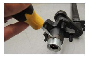
Once the cap is removed use the screwdriver to pry off the brass retaining ring.
