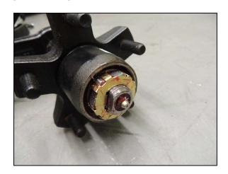
Use the hammer or rubber mallet to gently tap the aluminum cap on, ensuring that it is seated completely against the hub housing.
