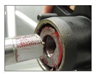
Ensure that the new hub is pushed all the way onto the shaft and that the washer and bearing are pressed in firmly. Install the nut, tightening it with the wrench, then loosen it slightly and snug it back down finger tight.
