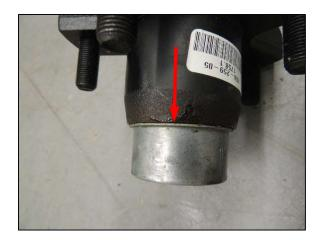
Press the rubber grease fitting cover on to the aluminum cap, taking care not to pinch the edges in.
