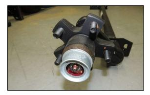
Use a hammer or mallet to dislodge the aluminum cap. Rotate the hub while tapping to help loosen. A screwdriver can be used as well to pry it free. Don't worry about damaging the cap as there is a replacement with your new hub.
