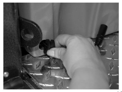
Push the plug back into the Grommet until the end protrudes about 1/4".
