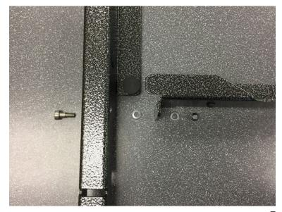
Set the mount assembly on the top of the GO pod below the bars as shown.
