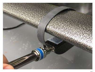
Tighten the nuts at all 4 connection points using your wrench/driver and hex wrench.
