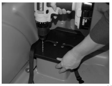
Install the **Flower Rivets** in each of the four holes to secure the Generator Mounting Plate in place.
