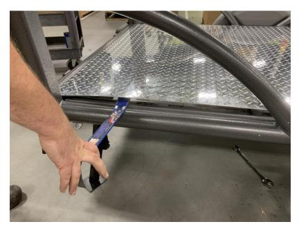
Remove the 3M tape residue. For best results, use an eraser wheel at its highest speed possible to remove the residue. If not all of the tape is able to be removed, that is alright. Be sure the surface is smooth and flat and there are not clumps. If there are clumps of tape, the deck will not sit flat.
