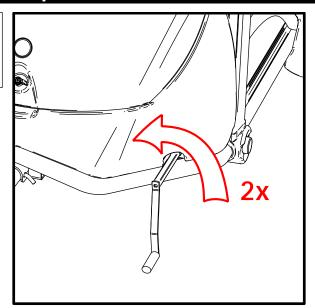
Rotate crank counter-clockwise two revolutions to allow the straps to hold the Rack and Tent Pod and relieve the load on the Lift Tubes.
