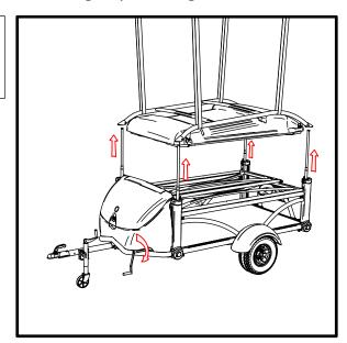
Carefully position the trailer beneath the suspended Rack and Tent Pod. Crank the Lift Tubes up until they are just beneath the Rack feet.
