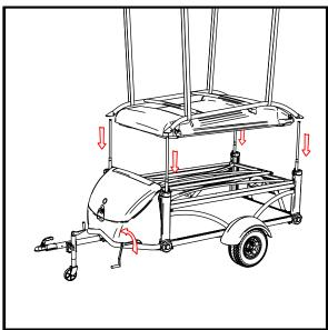
Continue to turn crank handle counter-clockwise while pushing Lift Tubes downward until they are flush with the top of the corner posts.
