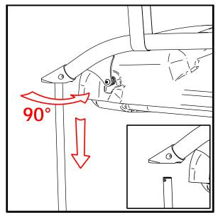
Rotate Lift Tube 90° and pull downward. Repeat for each corner of Rack.
