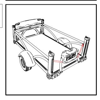
Secure the tailgate with a strap to ensure it remains upright during travel.
