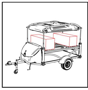
As an alternative to step 2, two sturdy boxes can be placed on the Bed Platforms as shown. The Tent Pod can be lowered onto the boxes to relieve the load on the Lift Tubes (as described in the next step).
