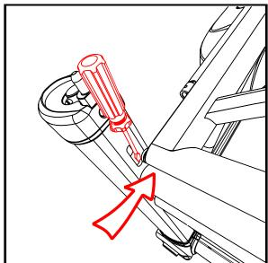
When the pin is fully retracted, push the Bed Platform frame inward to release the pin from the slot in the corner post.
