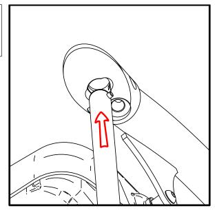
By hand, lift each Tube and push it into the Rack foot making sure that the pins are aligned with the tapered scallops on the edges of the hole. Do not twist.
