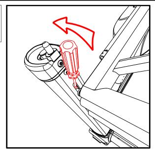
To remove Bed Platforms, use a flat screw driver to locate the retracing pivot pin on the Bed Frame. Usually, it is the end toward the rear of the trailer.
