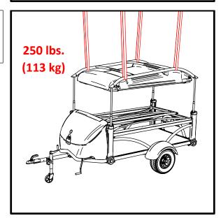
Attach straps to support Rack and Tent Pod. Straps must be able to safely support at least 250 lbs.
