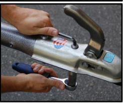
**Step 9**: Reinstall coupler on tongue extension using removed M12 bolts, washers and hex nuts. Tighten to 20 ft-lb (27 Nm).
