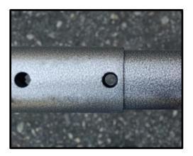
**Step 7**: Push the Tongue Extension in until the bolt holes on the bottom of the Tongue line up. It may be necessary to place a wooden block at the end of the Tongue Extension and hammer it to get it fully into place.
