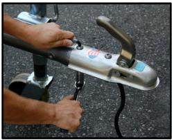
**Step 2**: Remove Coupler using 8mm hex key and 19mm socket wrench.
