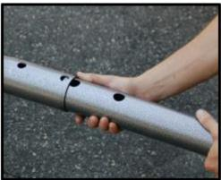
**Step 6**: Slide Tongue Extension into existing tongue (larger holes facing upward). Be sure the inside of the existing tongue is clean and smooth so the tongue extension will slide more easily.
