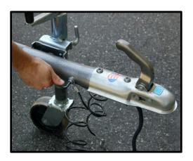
**Step 1**: Remove Safety Cables from tongue using 6mm hex key. Hex head bolt can be reinstalled in the holes rather than leaving the holes exposed if you prefer.
