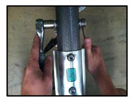
**Step 10**: Reinstall Safety Cables onto the Tongue Extension using M10 bolt, 2 washers, and M10 nut.
