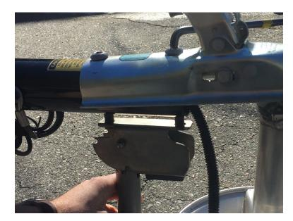
Ensure that both nuts are tight. The kickstand can be retracted by pulling down and then back.
