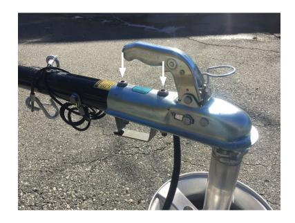
Use both wrenches to remove the nuts and washers on both bolts, and set the bracket aside.
