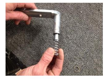
Reassemble the bracket by inserting the retractable pin, sliding the spring on top.
