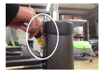
Using a flat head screwdriver, depress the retractable pin to release the bed frame and remove it from the side frame.
