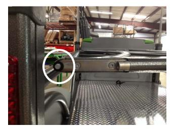
You will now be able to see the retractable pin and the plastic spacer that holds the bed frame in place.
