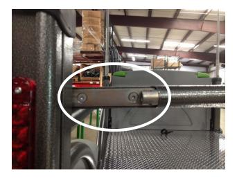
When the bed frame is lowered, you will see two hex bolts that attach the mounting bracket to the bed frame.
