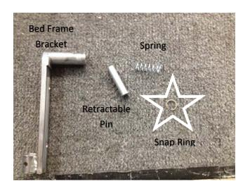
The disassembled bracket contains (in this order from the base) a retractable pin, a spring, and a snap ring.
