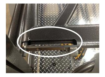
Using a 5 mm hex wrench, remove the bed frame bracket from the frame.
