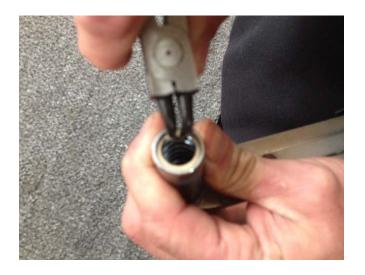
Using snap ring pliers reinstall the snap ring. There is a groove just inside the lip of the bracket where the snap ring should seat. Make sure the snap ring is fully secured within that groove.
