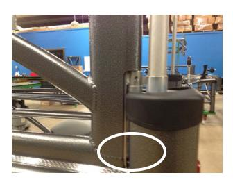
The bed frames attach to the side frame with a retractable pin, located on the bottom of the bed frame mounting bracket on the rear (step) side of the GO.
