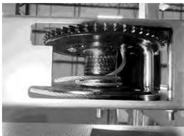
Has cable jumped outside of the spool?
