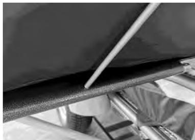
Orange pole attaches to bed support hole.
