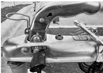
Coupler with indicator showing positive connection to ball.
