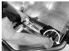
5. While keeping tension on the cable, respool cable back onto spool.
