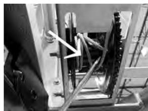
4. Once loose, unspool cable completely, or until the bind in the cable is gone.
