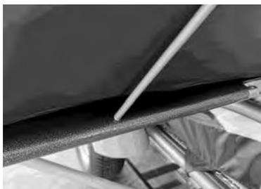
Vestibule pole inserted into frame hole.
