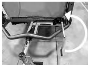
3. Using a flat head screwdriver and a twisting motion, relieve tension at the bind in the spool. **DO NOT USE FINGERS TO ATTEMPT CABLE UNTANGLING.**
