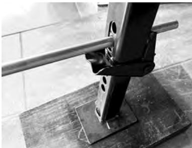
Stabilizer jack adjustment bar, passing through both sets of holes on stabilizer jack.
